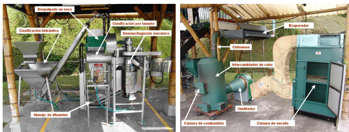
Figure 1a. Becolsub equipment to process 300 kg of coffee fruits per hour. Figure 1b. Mechanical dryer.
