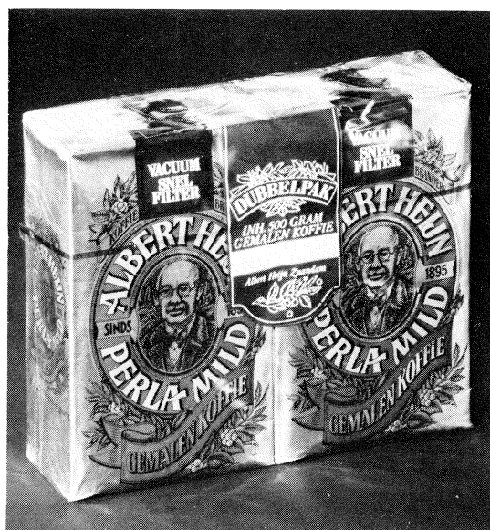
Fig. 11. — Two vacuum bags and a common regenerated cellulose wrapper (as per table I, item b)
