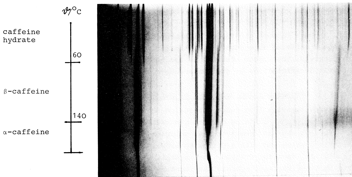
Fig. 1: X-ray diffraction pattern of caffeine as a function of temperature
