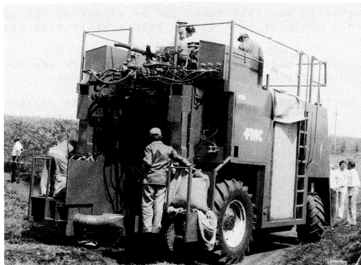
Fig. N o 2) Rear view of harvester turning into a row showing bagging-stations on each side.
