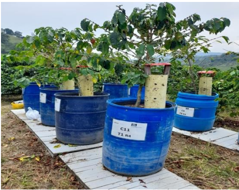
Figure 1: Lysimeters and volatilization chambers in the field study
