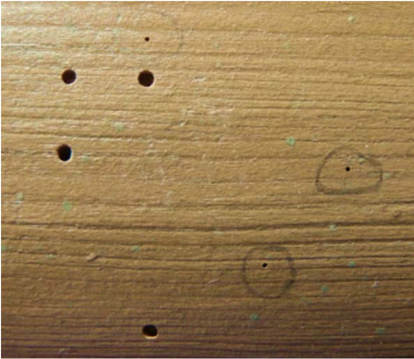
Figure 3: Exit holes of Anobium punctatum and Spathius exarator The exit holes of Anobium punctatum (about 2 mm) and Spathius exarator (about 0.5 mm; marked with a circle) are due to their differences in diameter clearly distinguishable and can be used as a measure for the monitoring of success.
